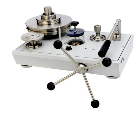
The Pressurements 3000 Series is the culmination of over 50 years experience in the production and design of primary pressure standards. With features designed to improve accuracy and performance, increase reliability and simplify operation these deadeweight testers can be used to calibrate virtually any pressure sensing device, including transducers, transmitters, gauges or pressure switches.
