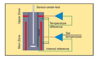
The calibrators of the RTC series allow a precise temperature calibration for a variety of sensor types and formats. This becomes possible through the innovative active dual zone heating block technology.
