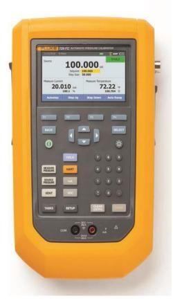
The Fluke 729 Automatic Pressure Calibrator has been designed specifically with process technicians in mind to simplify the pressure calibration process and provide faster, more accurate test results. Technicians know that calibrating pressure can be a time-consuming task, but the 729 makes it easier than ever with an internal electric pump that provides automatic pressure generation and regulation in an in an easy-to-use, rugged, portable package.
