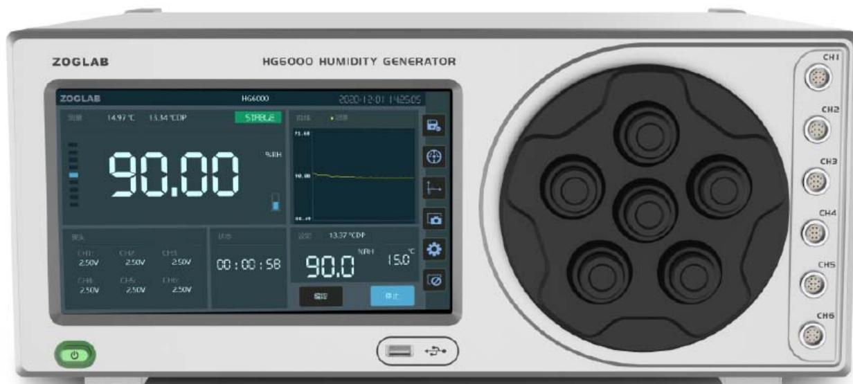
The EP-Z6000 line of humidity generators have a high capacity and uniformity and a 9 inch touchscreen display.
