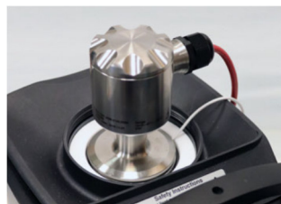
STS-102 A 035 sensor and sanitary sensor in an insert, mounted in an RTC-168 calibrator.
