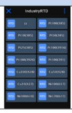
The ADT282 has an extensive built-in temperature sensor library, including ITS-90, CVD, Standard TC,13 types of industrial RTDs and 15 types of industrial thermocouples, and also supports sensor customization. The user can also edit the probe coefficients according to the ITS-90, CVD formulas and the R0 parameter of the industrial RTDs. The extensive probe library capabilities also support coefficient input methods for standard thermocouple types.
