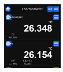
The model ADT282 includes dual inputs which provide support for a multitude of resistive type sensors (RTD's) as well as thermocouples (TC's). Both channels can be displayed simultaneously which allows for comparison measurements and a host of other statistical analysis capabilities. And the Additel 282 allows for easy differential measurement selection for T1-T2.
