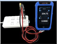
The Additel 226 non-Ex version is equipped with "true effective value" RMS measuring function, which can measure the RMS of various waveforms with no need to consider distortion or waveform parameters and other errors caused by various waveforms
